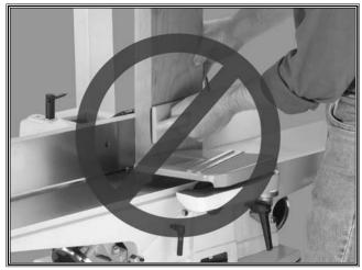
Figure 5. Never joint end grain!
